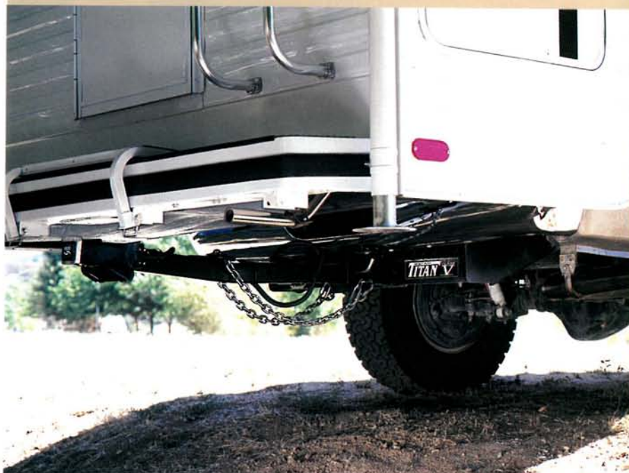
Reese TITAN Class V Receiver with 2 -1/2" steel tube extension bar.
